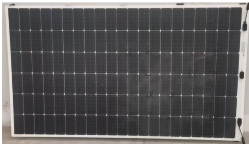
Sample 18#: Burning brand test (front)
